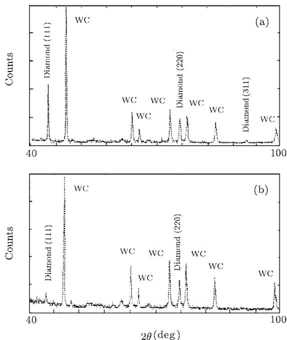
Fig. 2. XRD patterns of prism (a) and spherulitic (b) diamond film on WC-6%Co samples.
