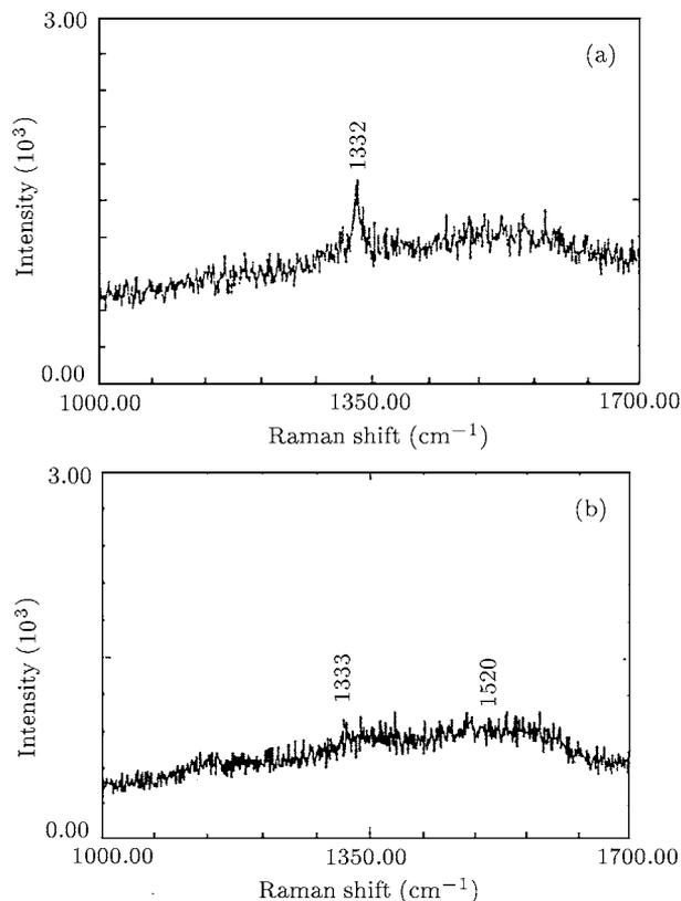
Fig. 3. Raman spectrum of the prism (a) and spherulitic (b) diamond films on WC-6%Co samples.
